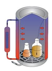
The LABOKLAV 55–195 series cooling system operates on the heat exchanger principle. Deionised water from the storage tank circulates through the double jacket, cooling the entire chamber before returning to the storage tank. There, it is cooled via a coil supplied with tap water.
