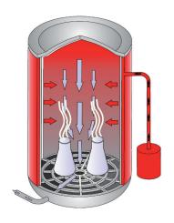
Vacuum drying with double-jacket heating, option V
